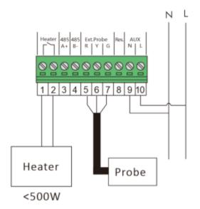
Optional wet node version, heater can be powered by the dehumidifier.
