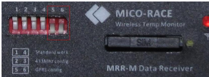
Change the PID switch 5.6 ON, as photo shown; and connect RS232 port to your host PC.
