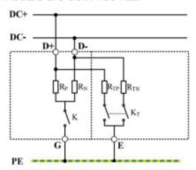
External self-test can detect whether the insulation monitoring circuit can work normally, whether the grounding switch K works reliably, whether the grounding point 'G' of the insulation monitoring is reliably connected to the ground wire, and whether the ground wire is reliably connected to the earth such as the ground bar or shell.
