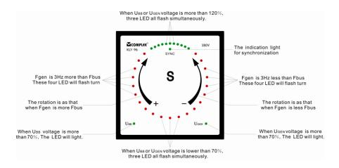
2.LED indicates the instant phase error  $\Delta \phi$ , the resolution ratio of red LED is 15°. The resolution ratio of green LED is 3° within the range of synchronized point ±15°. During normal operation period, only one LED lights among the circular bar graph will light, the position of LED is stimulated the actual phase angle difference. Details see below diagram:
